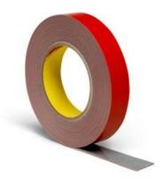
3M<sup>™</sup> Acrylic Foam Tape 5314 is a 0.76 mm (0.030 in) thick, gray, double-coated acrylic foam tape commonly used for the attachment of automotive exterior trim parts such as body side moldings.
