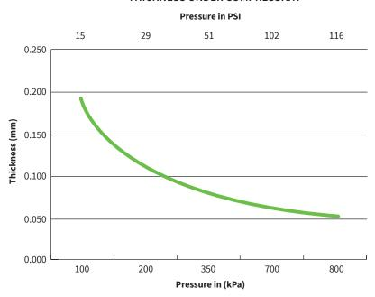
Material compressibility improves contact between the mating surfaces, adjusting for flatness and roughness variations, ensuring reliable performance.
