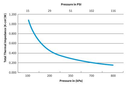
THERMAL IMPEDANCE VS. INTERFACE PRESSURE
