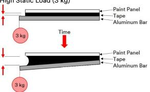
3M<sup>™</sup> Acrylic *Plus* Tape EX4011 demonstrates low elongation properties under low load conditions for good bond line aesthetics.
