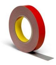
3M<sup>™</sup> Acrylic Foam Tape 5567 is a 1.52 mm (0.060 in) thick, gray, double-coated acrylic foam tape used for the attachment of a variety of automotive exterior trim parts.
