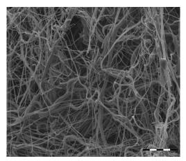
$\label{eq:magnified} \mbox{Magnified image of Thinsulate} \mbox{$^{\top}$M Acoustic Insulation showing} \\ \mbox{fine PP and larger PET fibres}.$
