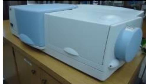
Sheldahl measures solar absorptance using a Perkin-Elmer Labsphere 950 UV-VIS-NIR spectrophotometer.
