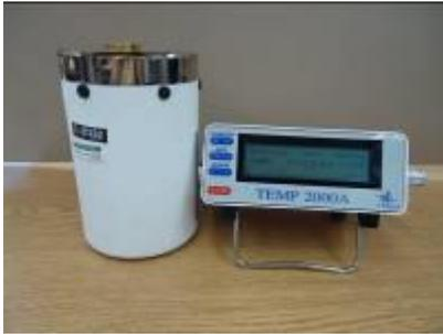
We can also test total normal reflectance on the AZ Technology Temp 2000A. A calculated normal emittance value can be provided by testing on the AZ Technology Temp 2000A Reflectometer in the Relative Mode. This meets ASTM-E408 Method B.
