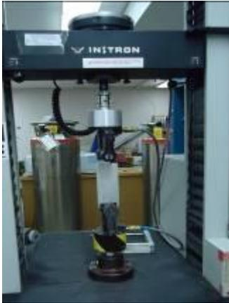
All tapes sold by Sheldahl are tested for bond strength. This test is done by applying the tape to a clean stainless steel substrate using a prescribed pressure and then measuring the force required to remove the tape using an Instron instrument. Our test methodology is in accordance with ASTM D-1000 and ASTM D-3330. We can also test adhesion to aluminum plates if desired.
