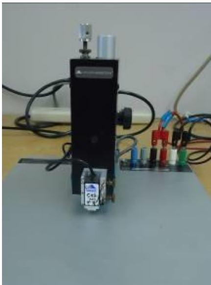
When small test samples are available, or we cannot cut a test sample for surface resistivity testing we use a four point probe as described in Q000322.
